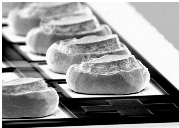
Figure 7: Ball bumps wire bonded on a silicon die
